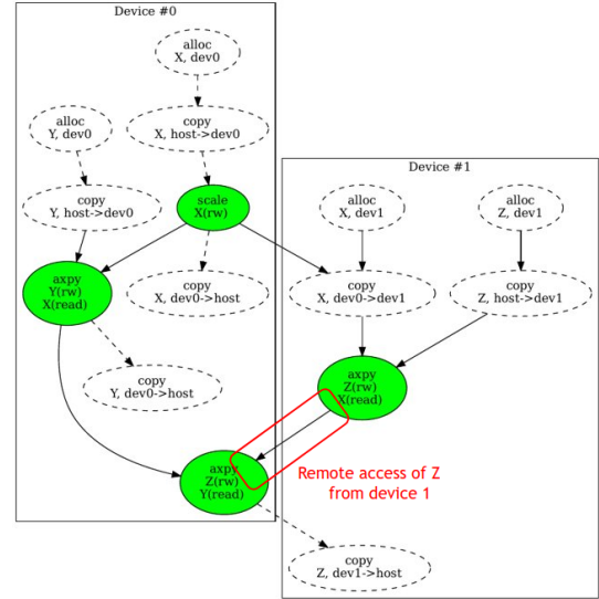
Fig. 1: Task graph obtained with code on Figure 2 when using places (high level tasks are depicted in green, ancillary tasks have dotted contours)
